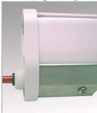
Figure 9. Gas Line Plug
