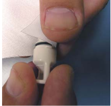
Figure 11. Lightly coating o-rings on nozzle with lubricant.
